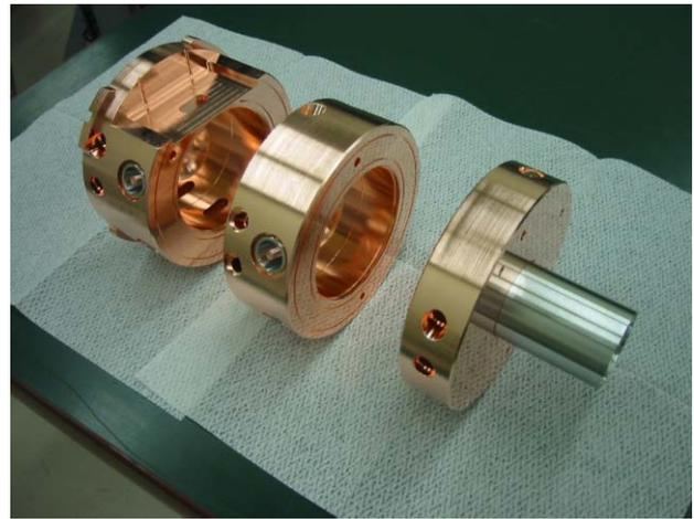
Figure 4: The cells with the new tuners before brazing.
