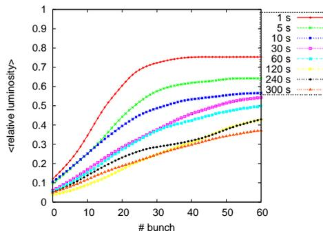
Figure 3: Beam-based IP position feedback simulation for the  $e^+e^-$  collision with ground motion model B applied during different times along the BDS. The average relative luminosity is calculated over 50 seeds.
