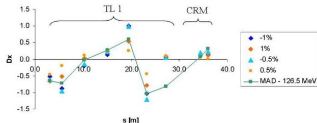
Figure 2: Dispersion measurement in TL1 and ring injection region. (The difference at the end of TL1 ( $s=27$  m) is due to a defective pick-up.)
