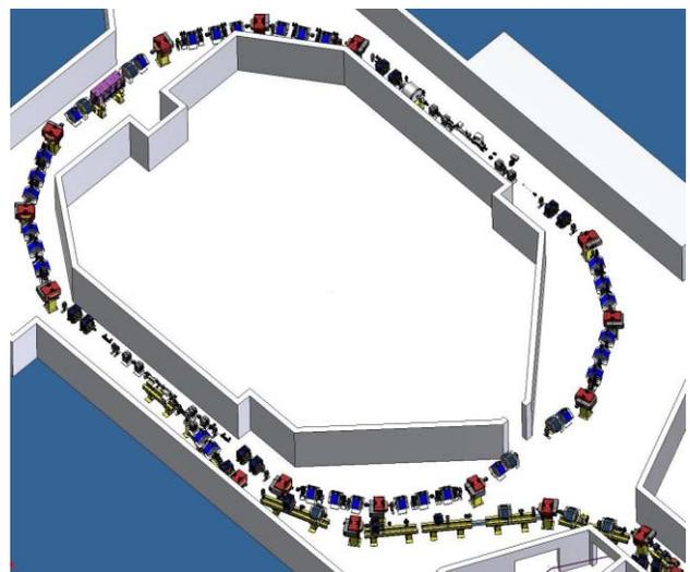
Figure 1: Layout of the TL1 transfer line and the combiner ring. The beam arrives after the delay loop (not visible) from the bottom right into TL1.
