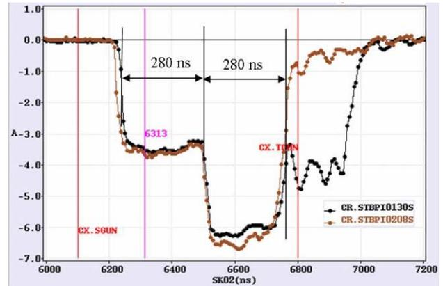
Figure 3: First recombination in the Combiner Ring. The traces show the beam current measured by 2 beam position monitors. The incoming beam pulse has twice the length of the CR ( $2 \times 280 \text{ ns}$ ). During the second 280 ns, the bunches are interleaved with the bunches that made one revolution in the ring.
