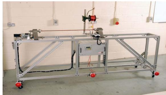
Figure 3: A test winding of 1-m long undulator prototype on a custom built winding machine.
