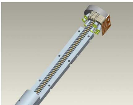
Figure 1: Conceptual design of the helical undulator section.
