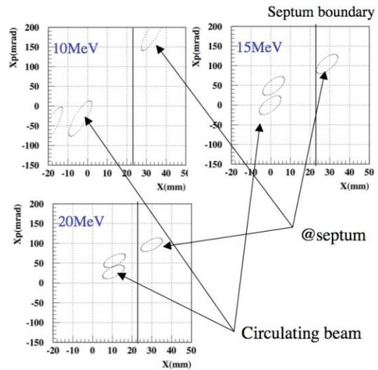
Figure 2 Phase space distribution of the injected beam of a typical operation mode
