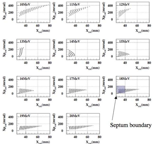
Figure 3 Beam center distributions in the phase space at the injection septum of a typical operation mode. The shaded region in 18MeV is that in common among all the investigated injection conditions
