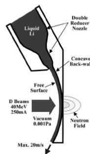
Fig. 1. Concave liquid flow for the IFMIF target [1].
