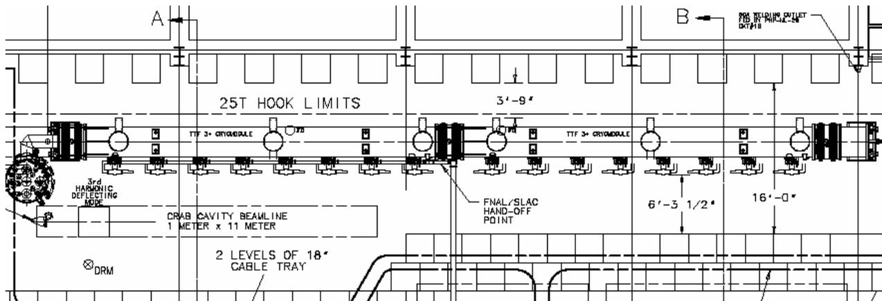
Figure 2: Two RF cryomodule acceleration section for ILCTA.
