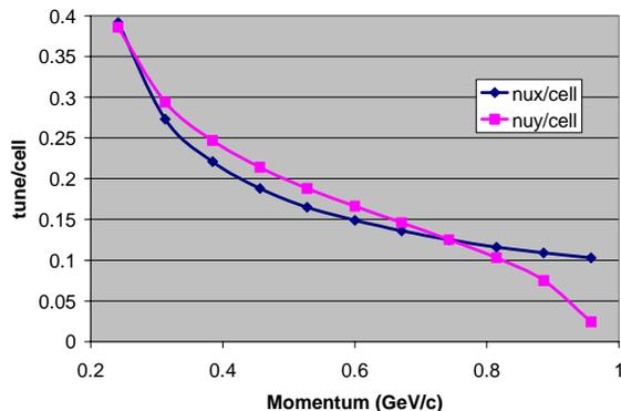
Figure 2. Dependence of cell tune on momentum in a nonscaling, linear-field FFAG designed for muon acceleration.
