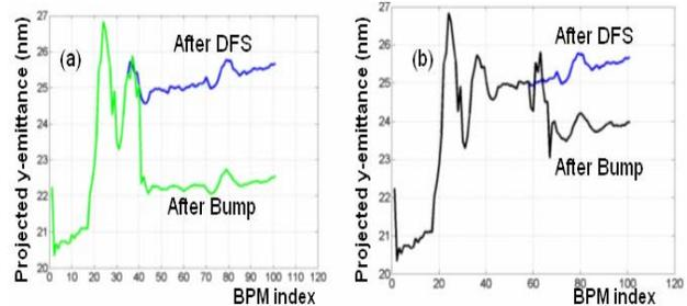
Figure 4: Average projected emittance growth in a nominally misaligned linac for 30 seeds after dispersion free steering, and then implementing a dispersion bump (a) at corrector no. 36, and (b) at corrector no. 59.
