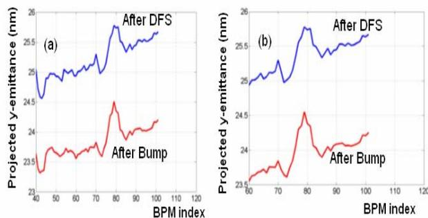
Figure 6: Average projected emittance growth in a nominally misaligned linac for 30 seeds after dispersion free steering, and then implementing one wakefield bump (a) at corrector no. 3, and (b) at corrector no. 39.
