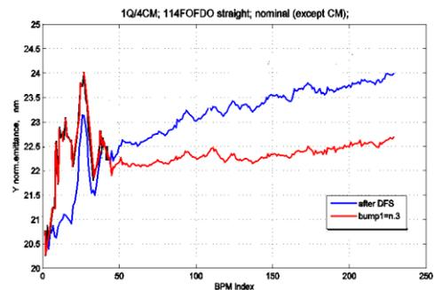
Figure 8: Average projected emittance growth in a nominally misaligned linac for 30 seeds after DFS, and then implementing one dispersion bump at corrector no.3.
