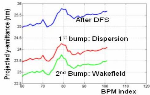
Figure 7: Average projected emittance growth in a nominally misaligned linac for 30 seeds after DFS, and then implementing one dispersion bump at corrector no.3, and one wakefield bump at corrector no. 39.
