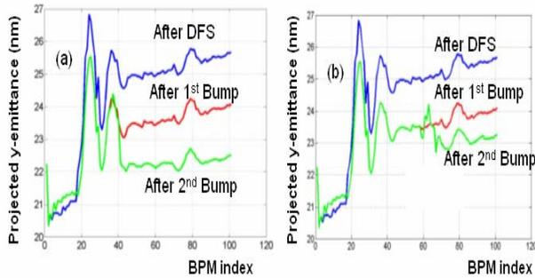
Figure 5: Average projected emittance growth in a nominally misaligned linac for 30 seeds after dispersion free steering, and then implementing two dispersion bumps (a) at corrector no. 3 and 36, and (b) at corrector no. 3 and 59.
