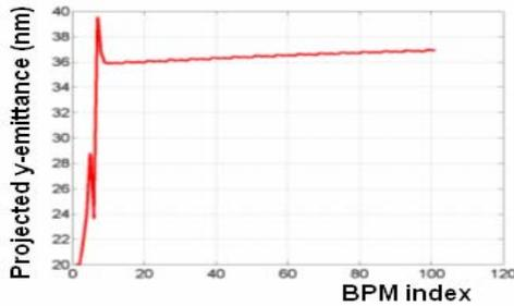
Figure 1: Projected emittance growth due to an excited dispersion bump placed very close to the main linac entrance in an otherwise perfect linac.
