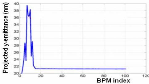
Figure 2: Projected emittance growth due to an excited wakefield bump placed very close to the main linac injection in an otherwise perfect linac.
