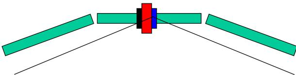
Figure 3: Curvature implementation. Green blocks are cryomodules, black block is the BPM, red - quadrupole, blue - corrector, black line is the beam orbit.
