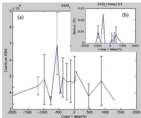
Figure 2: (a) Measured total charge by the beam phosphor screen (BPS), which consists of a phosphor screen (Lanex fast, Kodak), and a CCD camera, against the timing delay of Collider beam. (b) Measured neutron yield against the timing delay of the Collider beam.
