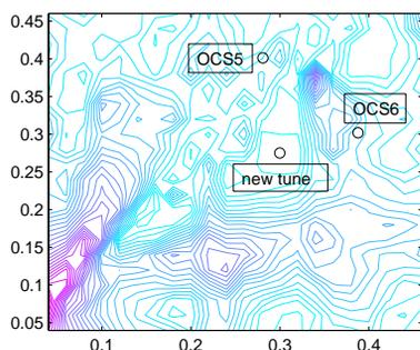
Figure 5: Tune diffusion rates for different tunes.
