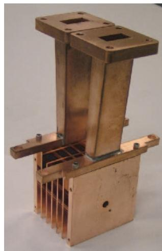
Figure 2: 6 cell metallic PBG accelerator structure
