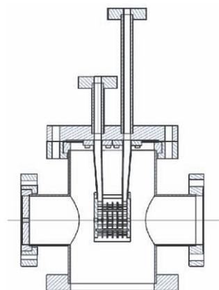
Figure 3: PBG accelerator structure vacuum vessel
