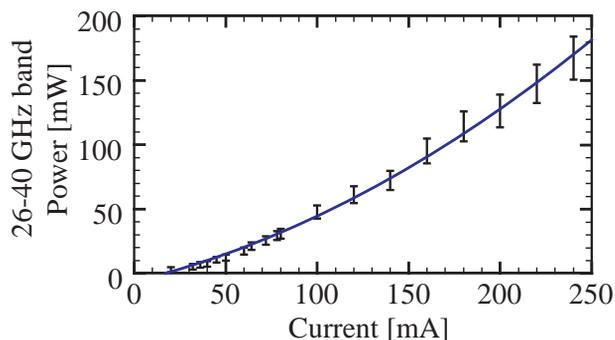
Figure 4: Scaling of power in Ka (26-40 GHz) band with current. Quadratic fit shown in blue with data given as black bars
