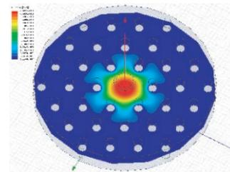
Figure 1: HFSS simulation results showing the electric field magnitude of the  $TM_{01}$ -like fundamental operating mode of the PBG accelerator structure. Simulation parameters are as listed in Table 1.
