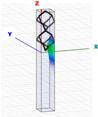
Fig. 3. Simulation of surface mode on the interface of the diamond wire lattice.
