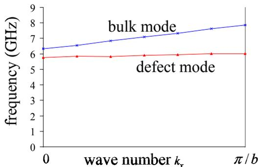
Fig. 7. Dispersion of plasmonic waveguide modes. The defect mode is an accelerating mode. The cubic cell length  $a=2.3$  cm, wire radius  $r=0.07$  cm.
