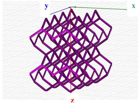
Fig. 1. Metallic photonic crystal built as a diamond lattice of intersecting wires.
