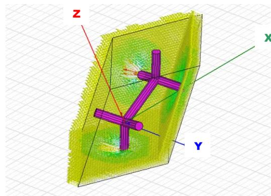
Fig. 2. Simulation of bulk modes in the diamond wire lattice using the primitive cell. A longitudinal plasma mode at 6.25 GHz is shown for the lattice cubic cell length  $a=2.3$  cm and the wire radius  $r=0.07$  cm.
