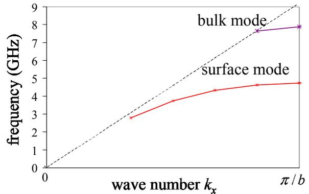
Fig. 4. Dispersion of surface waves on the interface of the diamond metallic lattice. The cubic cell period  $a=2.3$  cm, wire radius  $r=0.07$  cm. The dashed line depicts the light cone.
