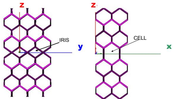
Fig. 5. Accelerator structure using a defect in 3D metallic diamond wire lattice. An electron beam traverses in the  $x$ -direction.
