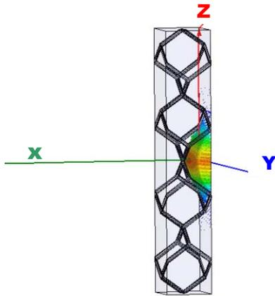
Fig. 6. Simulation of plasmonic waveguide. The defect mode is a longitudinal TM-like mode propagating in the  $x$ -direction. The electric field distribution is shown.
