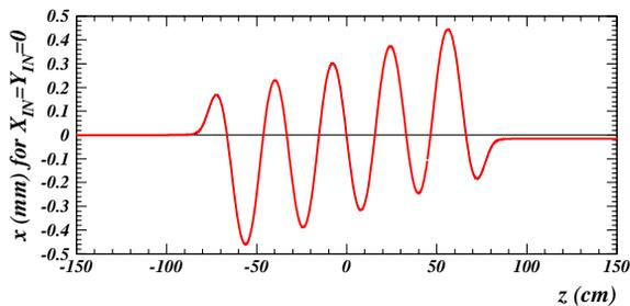
Figure 4: Trajectory in the horizontal plane for 5 GeV electrons of perpendicular incidence on the symmetry axis of the wiggler.
