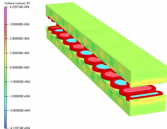
Figure 1: 12-pole optimized damping ring wiggler. The color scale on the surface of the model shows the magnitude of the vertical magnetic field component.
