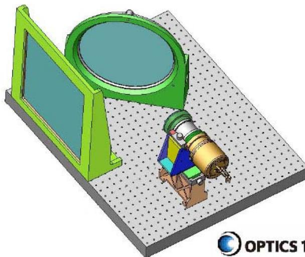
Figure 7: Conceptual drawing of the integrated imaging system showing the camera/lens assembly, turning mirror, and scintillator in its holder. Not shown is the light tight enclosure surrounding the components.
