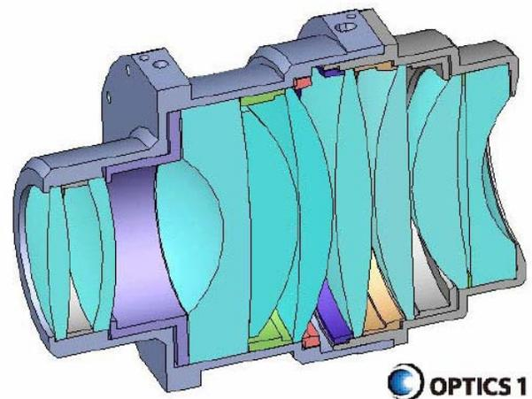
Figure 4: Drawing showing the 9 lens elements in the assembly. The entrance aperture is on the left.
