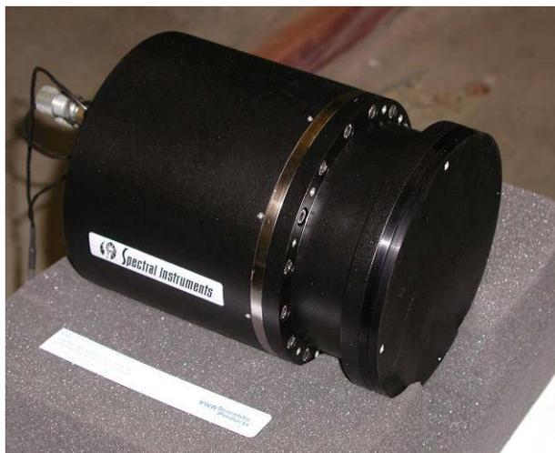
Figure 6: A photo of the 4096 x 4096 (15 micron) pixel cryogenically-cooled 1100 Series CCD camera built by Spectral Instruments. The nom. 6" diameter entrance aperture on the right will be close-coupled to the lens.
