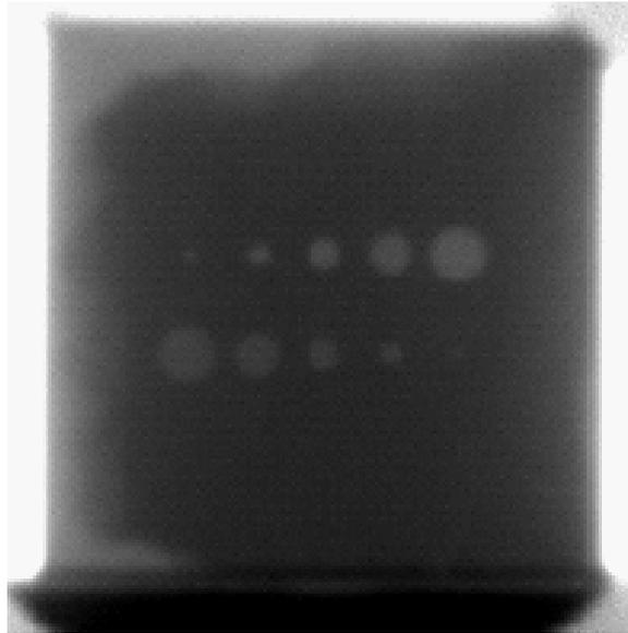
Figure 2: A fast neutron radiograph of 1” thick LiD block shielded by 2” of depleted uranium. The image shows not only the test holes drilled down to cubic mm void size, but also showed where material around the edges cracked off during machining.
