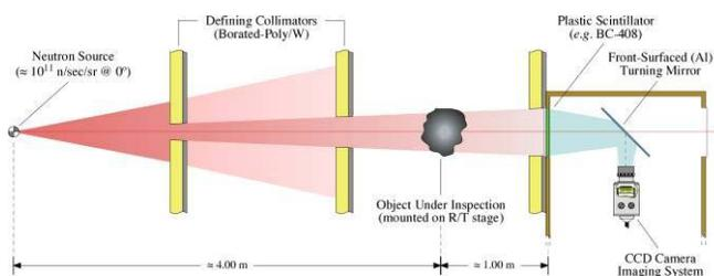
Figure 1: A layout for doing fast neutron imaging, showing the neutron source as the dot on the left, and the neutron beam as it is collimated before creating a shadow radiograph on a scintillator on the right. The light is then turned with a mirror and focused onto the CCD camera using a wide-aperture fast lens.
