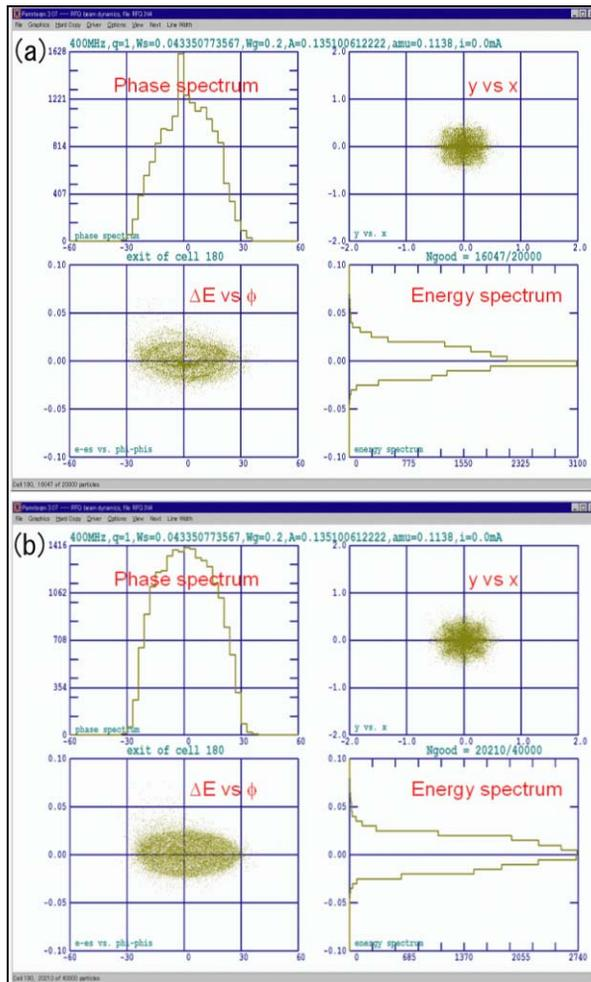
Figure 5: Phase, spatial and energy distributions of muon beam after acceleration with initial beams of (a) monochromatic 20 keV and (b) 20 keV,  $\Delta E = 5$  keV.
