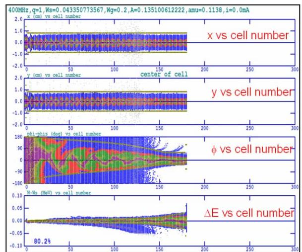
Figure 4: PARMTEQ beam transport simulation in RFQ-A. Parameters of the RFQ is on Table 1.
