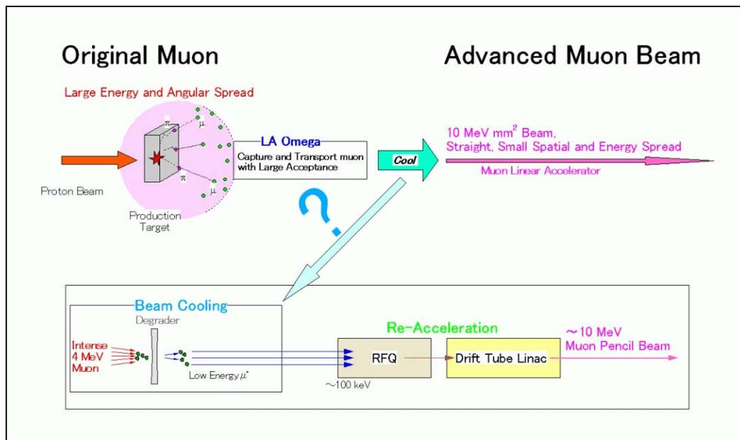
Figure 1: Schematic diagram of advanced-muon-beam generation.
