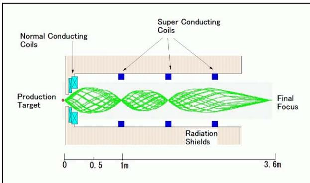
Figure 2: Schematic view of LA Omega muon channel.
