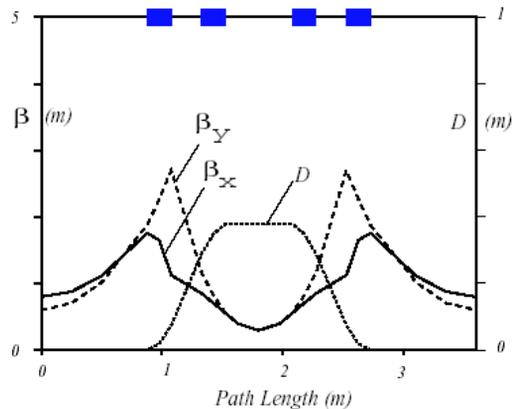
Figure 3:  $\beta_x$ ,  $\beta_y$  and  $\eta$  as a function of  $z$  in a 45 degree bending cell.
