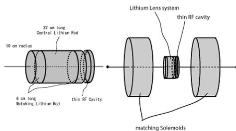
Figure 6: A schematic diagram of a Lithium lens (left) and straight section (right).
