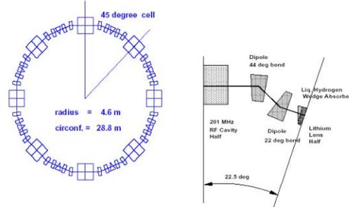
Figure 2: A top view of a muon cooling ring and a schematic diagram of a half of 45 degree bending cell.
