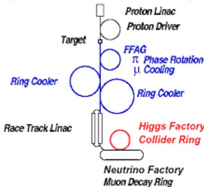
Figure 1: A schematic diagram of a  $\nu$  factory and a  $\mu^+ \mu^-$  collider.
