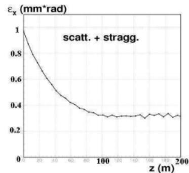
Figure 8: Normalized transverse emittance as a function of  $z$  through 33 sets of straight sections.
