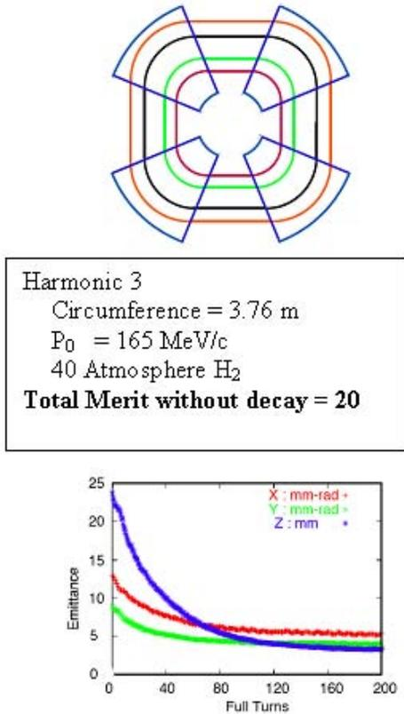
Figure 4: 4-dipole ring: schematic diagram, parameters and performance for harmonic number 3.
