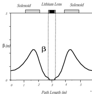
Figure 7:  $\beta$  as a function of  $s$  in the Lithium lens and matching cells with solenoids
