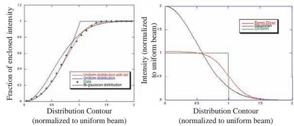
Figure 4: Analysis of streak data, with fraction of integrated intensity of data inside of elliptical contour shown. Best fit of data points to three models are shown: bi-gaussian distribution, uniform elliptical distribution, and Fermi-Dirac (uniform with tails) distribution.
