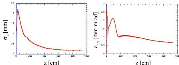
Figure 2: (left) Evolution of RMS transverse beam size  $\sigma_x$  and (right) evolution of RMS normalized emittance  $\epsilon_{n,x}$  for emittance compensation case, from *parmel*a simulation.
