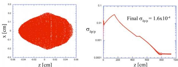
Figure 1: (left) *parmel*a simulation results of electron bunch  $(x, z)$  distribution showing ellipsoidal bunch boundary, and (right) evolution of  $\sigma_{\delta p/p}$  in  $z$  for emittance compensation case.
