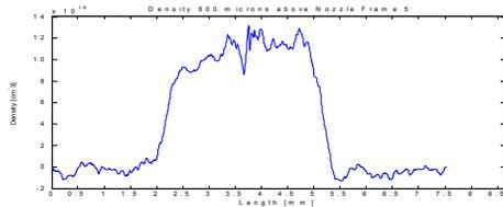
Figure 2: Neutral density profile of a 3mm Supersonic Nozzle at a distance of 800 microns.
