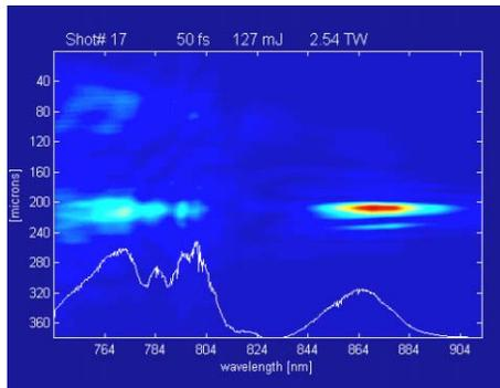
Figure 6: Data showing characteristic red shift (photon deceleration) from self phase modulation in the plasma wake.
