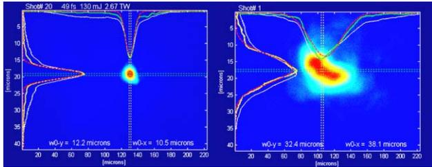
Figure 5: Images of the laser spot. The left image shows the self-guided 2.5 TW laser beam at the exit of a nominally 2mm long plasma with a density of  $1.5 \cdot 10^{19} \text{ cm}^{-3}$ . The image to right shows the beam imaged at the same location with no gas jet.
