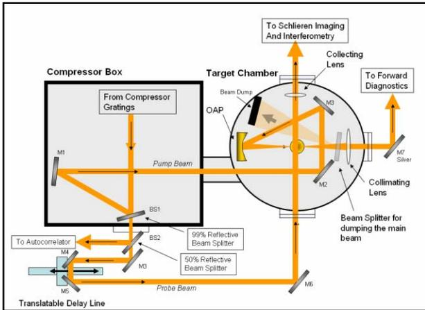
Figure 1: Experimental Setup showing the vacuum compressor, the target chamber and probe delay line, OAP, and beam dump.
