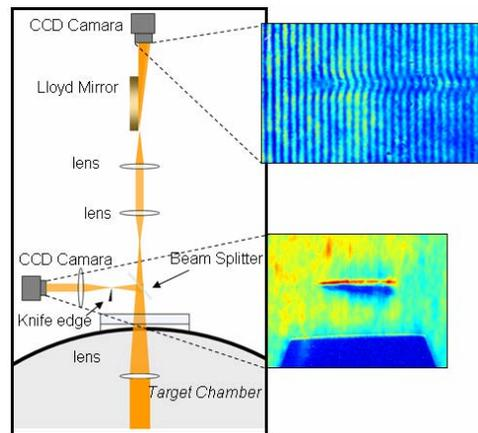
Figure 3: Diagram of the probe diagnostic setup showing Schlieren imaging and Lloyd mirror interferometry.
