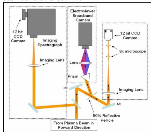
Figure 4: Schematic diagram of the forward diagnostic setup showing the imaging spectrometer, the prism spectrometer and the microscope for imaging the spot.
