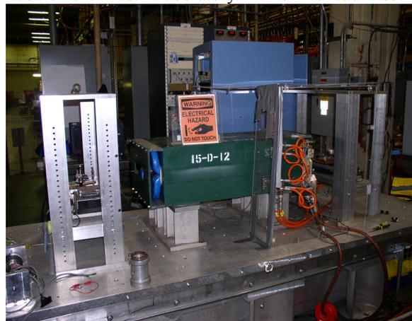
Figure 2: 10D37 dipole magnet on the test bench.
