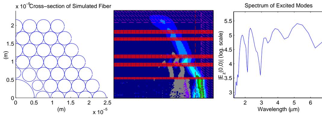
Figure 2: Left: Approximated cross-section of HC-1550 used in simulation. Center: Snap-shot of  $E_z$  field produced by beam traversing fiber. Right: Resulting spectrum excited by the electron beam.
