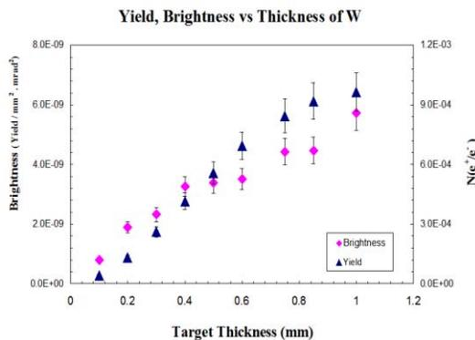
Figure 2: Brightness and positron efficiency depending on target thickness.
