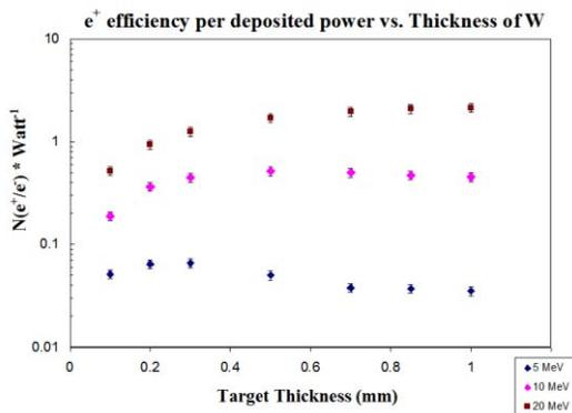
Figure 1: Positron production efficiency per deposited power in the target, as a function of target thickness. Three values of the incident electron energy are shown.
