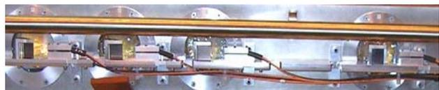
Figure 4: Fiber bundles and optic components.
