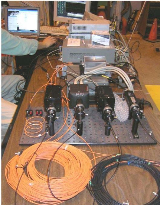
Figure 5: High-speed cameras and laser equipment.
