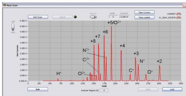
Figure 5: Control screen of the mass scan utility, showing an unoptimized Ar charge state distribution.
