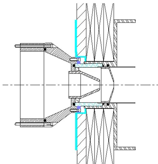
Figure 2: HV insulation of the source extraction region, showing the two added Delrin insulators (solid colors). The main extraction insulator is indicated by blue zipping.
