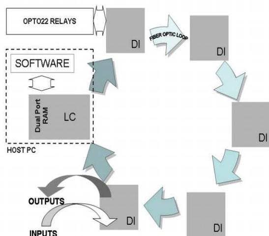
Figure 3: Caprice ECR/Floating beam line control system network diagram. Communication between the host PC loop controller (LC) and the device interfaces (DI) is via fiber optic cables.
