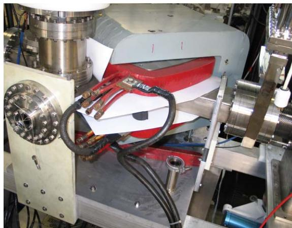
Figure 1: HV insulation of the main analyzing magnet.
