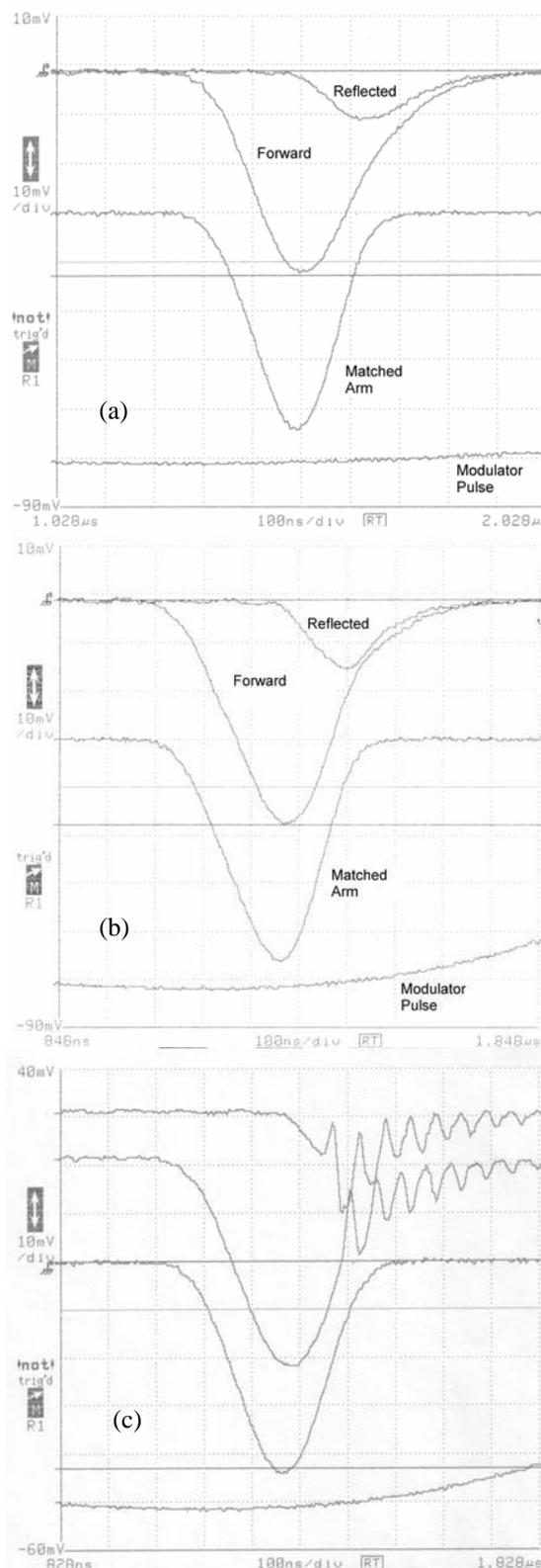
Figure 3: Forward and reverse power in gun arm and forward power in orthogonal arm of magnicon for a) long modulator pulse, b) short modulator pulse, and c) showing a breakdown event. Note in (c) that the matched, orthogonal magnicon arm is not affected by the breakdown in the gun.
