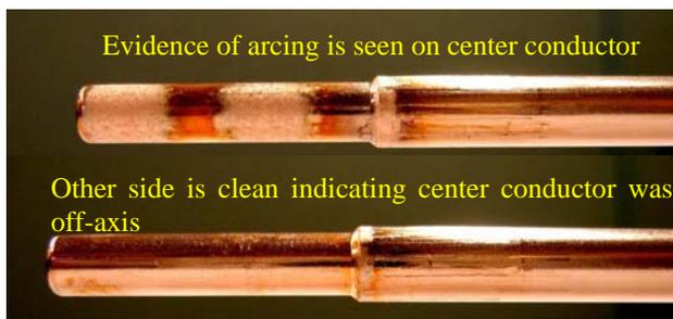
Figure 5: Photos of center conductor after conditioning.
