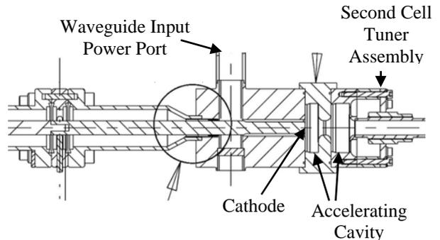
Figure 1: Cross-Sectional View of Gun Assembly
