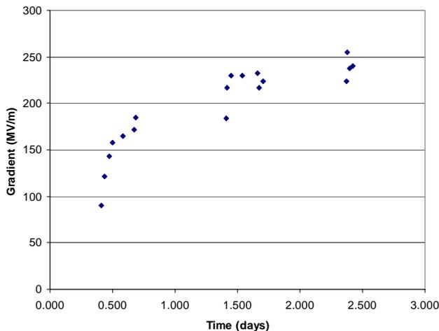
Figure 4: Conditioning history of gun showing calculated gradient as a function of time.
