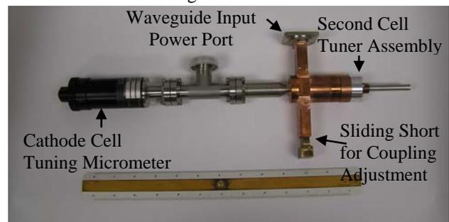
Figure 2: Gun cold model assembly.
