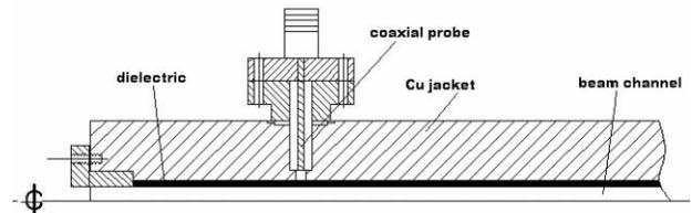
Figure 2. Part of the 26 GHz dielectric-loaded accelerating structure for the wakefield transformer ratio enhancement experiment.
