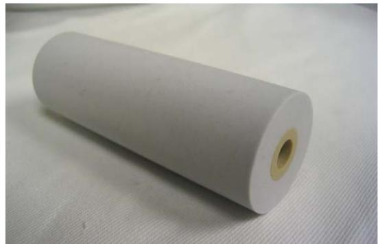
Figure 1: Double layered ceramic tube for the X-band dual layer DLA structure.
