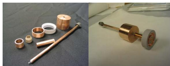
Figure 4: The fabricated  $TM_{03}$  mode launcher for the bench test of the dual layer DLA structure: components (left) and assembly (right).
