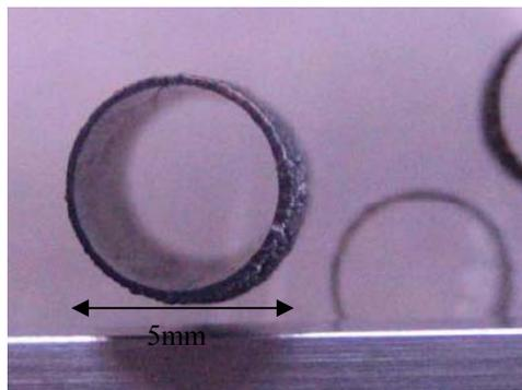
Figure 1: End view of the completed 0.5 mm wall 34 GHz diamond tube.
