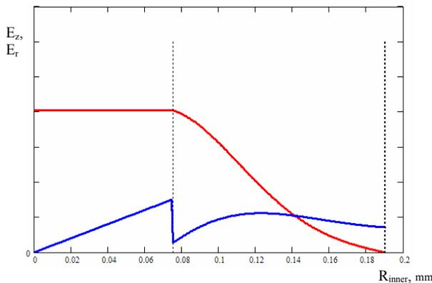
Figure 4: Longitudinal (red) and transverse (blue) electric field profiles normalized to the acceleration gradient  $E_{\text{accel}}$  for the structure parameters: (a) - ID 1.5 mm, OD 3.79 mm, thickness 1.15 mm.
