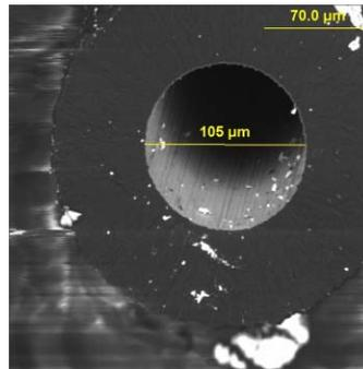
Figure 3: SEM cross-sectional surface images of a hot filament diamond tube of 105- $\mu$ m diameter, 70  $\mu$ m wall thickness.
