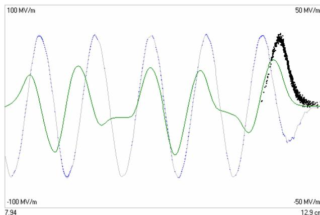
Figure 5: Wakefields (longitudinal: blue, transverse: green) and beam profile for the Ka band dielectric wakefield experiment.
