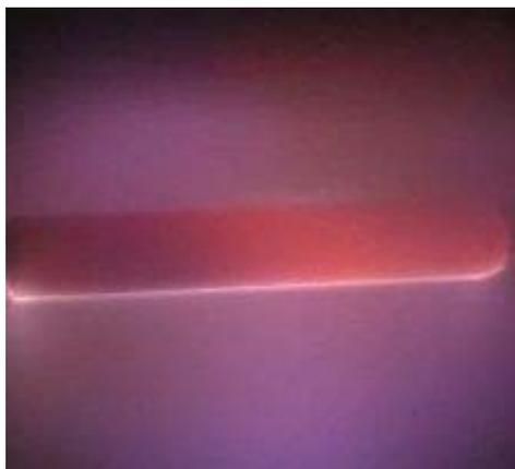
Figure 2: Photograph of the 5 mm ID diamond tube growing in the PECVD reactor.
