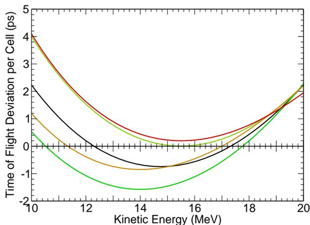
Figure 4: Time of flight as a function of energy for lattices where the minimum in the time of flight is moved to either 14 MeV or 15.5 MeV. The RF frequencies are identical in all cases.
