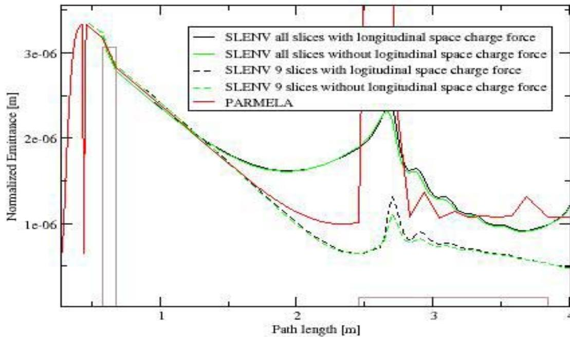
Figure 2: Beam Emittance calculated with PARMELA and SLENV in different modes.
