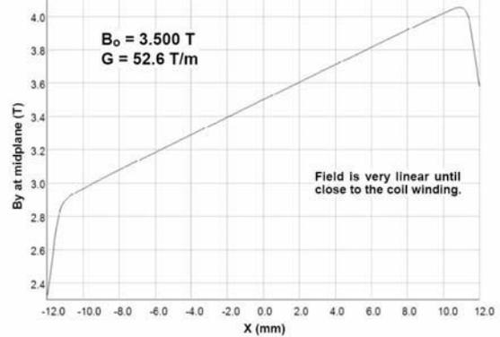
Figure 9: Magnetic field along the transverse axis.
