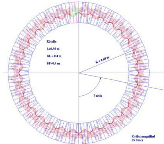
Figure 3: Non-scaling FFAG ring to be used for the gantry design. Orbit offsets are magnified 25 times.
