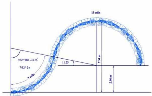
Figure 4: A gantry made of 7 and 15 cells of the ring presented in previous figure. Orbit offsets are magnified 25 times. Tracking is performed with the PTC program.
