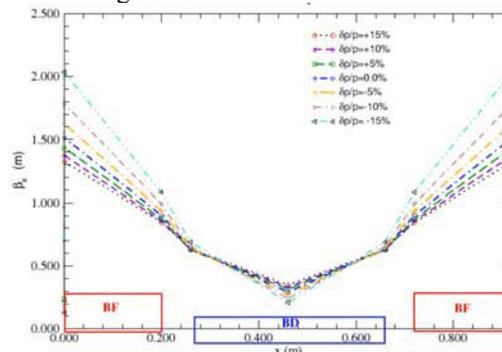
Figure 1: Betatron functions in one gantry cell.
