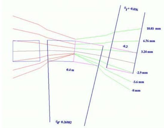
Figure 2: The basic cell of the gantry made of non-scaling FFAG combined function magnets.
