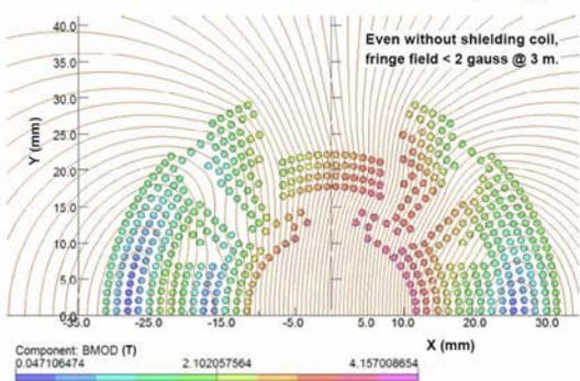
Figure 8: Preliminary superconducting combined function magnet design.
