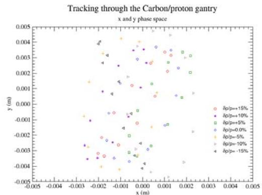
Figure 6: Tracking results in the  $x$ - $y$  plane.
