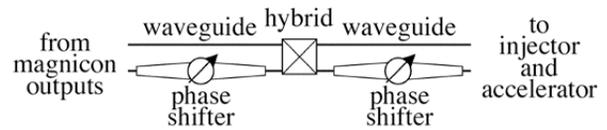
Figure 5: Schematic of the power combiner assembly.
