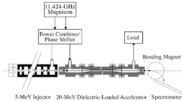
Figure 2: Schematic diagram of a dielectric-loaded test accelerator.
