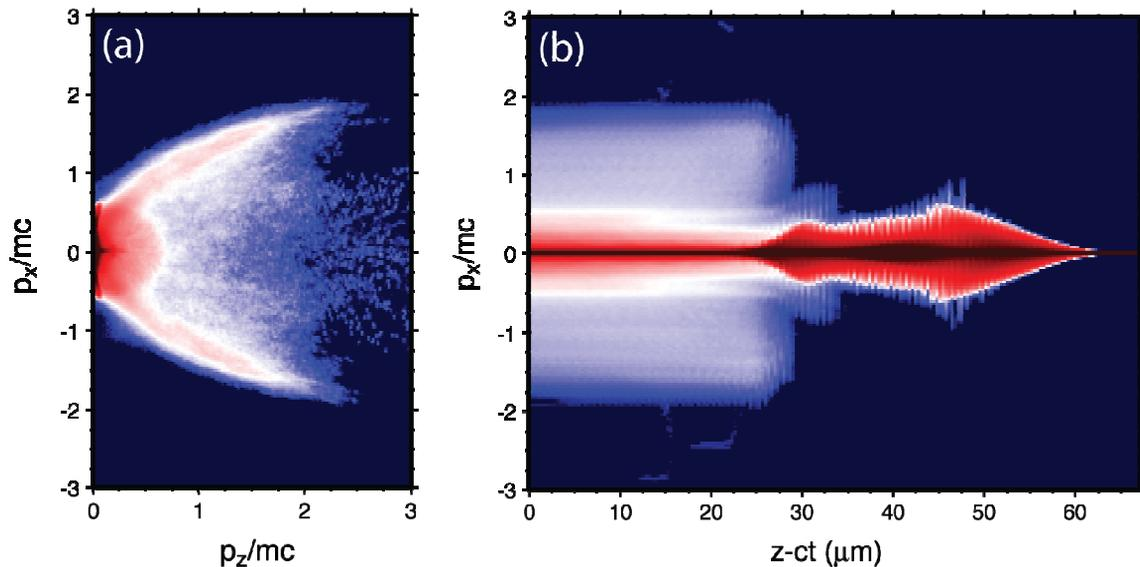
Figure 5: Time integrated phase space plots of electrons outside the laser focus showing (a) high density of particles at 45 degree propagation angle and (b) electrons at the quiver momentum appearing behind the laser pulse. The laser energy is predominantly in the region between  $z-ct = 30$  and  $z-ct = 50$ . The color map is referenced to a log scale.
