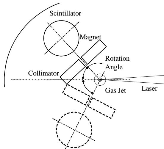
Figure 1: Experimental system with rotational arm electron spectrometer.
