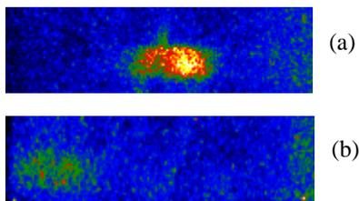
Figure 3: Scintillator images at 40 degree of electron spectrometer setup. No magnetic field (a), 0.2 kG (b).
