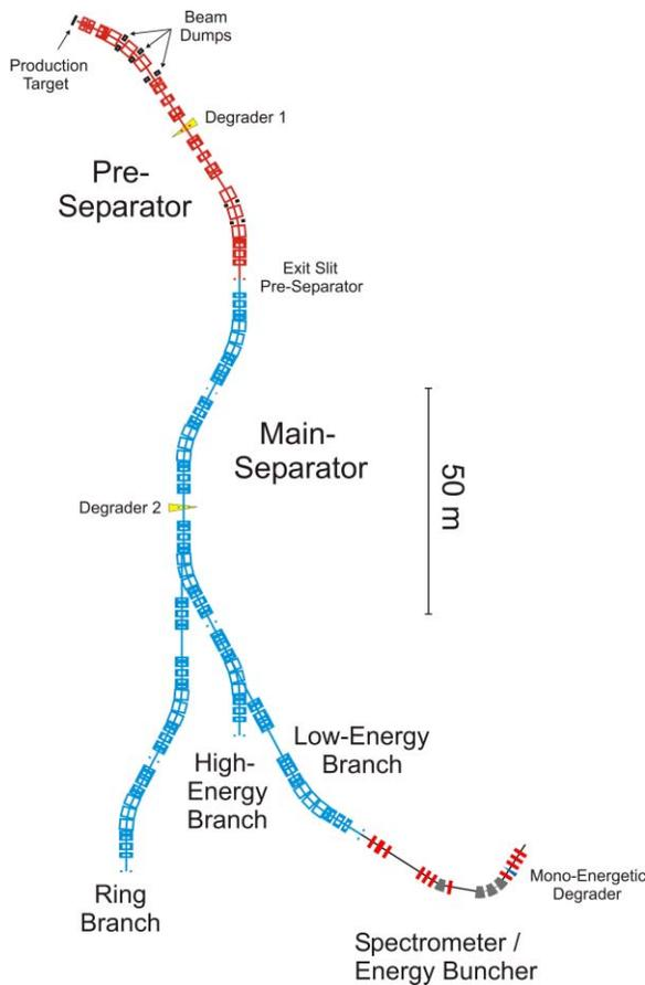
Figure 4: Layout of the Super-FRS for the production, separation and investigation of exotic nuclei. Separated rare isotope beams are delivered to three branches.
