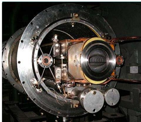
Figure 3: Photo of the original NUCLOTRON dipole.
