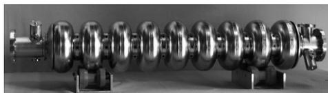
Fig. 1: A TESLA 9-cell cavity with a length of about 1m.
