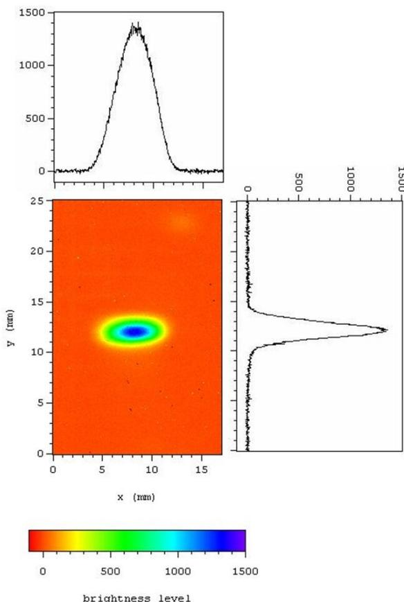
Figure 10: CCD Image Post Processed with jet measured as 6.5mm FWHM in x-axis and 1.6mm FWHM in the y axis. The camera has a full 16-bit (65535) brightness level [9].
