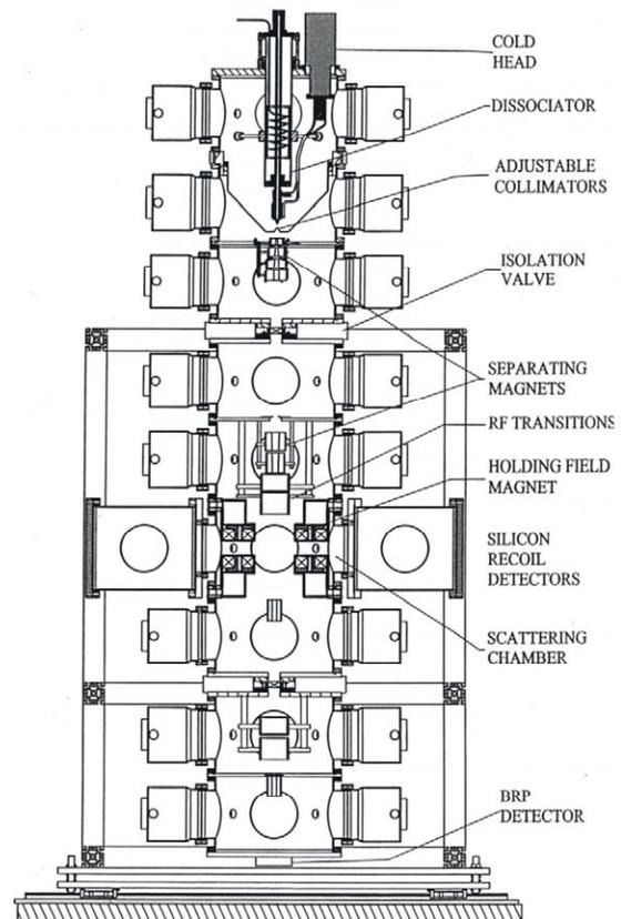
Figure 1: Hydrogen jet polarimeter layout.
