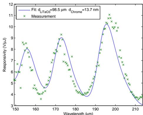
Figure 2: Response of a pyroelectric detector. The fit describes absorption in a stack of a thin Chrome top electrode, a  $\text{LiTaO}_3$  crystal and a thick gold back electrode. The optical constant of  $\text{LiTaO}_3$  are not known precisely, limiting the quality of the fit.
