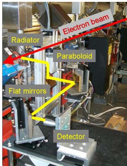
Figure 3: Bunch compression monitor setup at FLASH.
