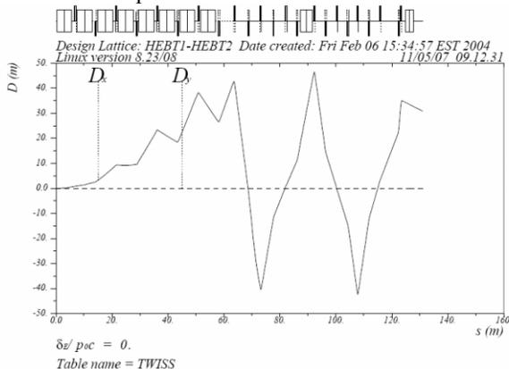
Figure 4: Dispersion function in the HEBT. The interaction point is at  $s=84$  m.
