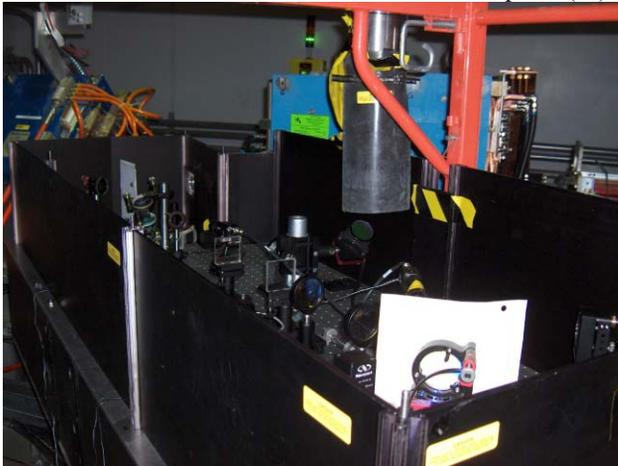
Figure 2: Laser beam optics that transfers the beam from the laser to the center of the magnet assembly through a flange window seen at the far end of the optics table.
