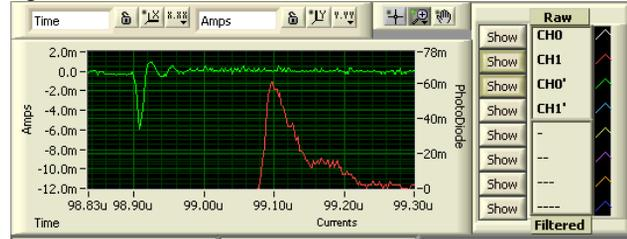
Figure 3: Laser stripping signal from current transformer (green) and reflected laser light signal from photodiode (red) used as a time reference point. The vertical scale is in milliamperes, the horizontal scale units are microseconds. The current pulse width is about 10 ns, which is slightly larger than that of the laser pulse. Photodiode signal time is shifted 200 ns from the current signal due to cable delay.
