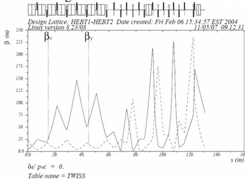
Figure 5: Horizontal and vertical betatron functions in the HEBT. The interaction point is at  $s=84$  m.
