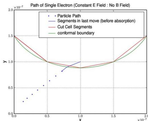
Figure 1: Trajectory of a particle being removed at a cut cell boundary
