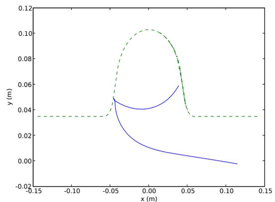
Figure 4: Multipacting trajectory of electron on a plane parallel to the cavity axis. This trajectory exits out the beam pipe. The cavity wall is shown as a dashed line.
