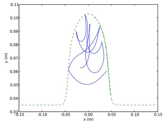
Figure 3: Multipacting trajectory of electron on a plane parallel to the cavity axis. This trajectory remains inside the cavity cell. The cavity wall is shown as a dashed line.
