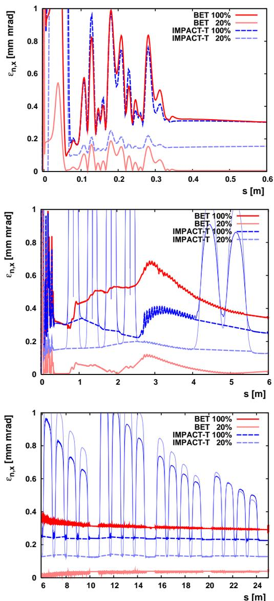
Figure 2: Projected and 20% slice emittance in the two-cell capture cavity (top), up to the end of the L-band structure (middle) and in the S-band structure (bottom).
