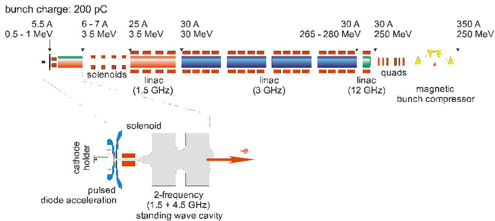
Figure 1: Overview of the 250 MeV linac (top) with a detailed sketch of the first accelerating elements (bottom). Target beam currents and energies along the machine are indicated.
