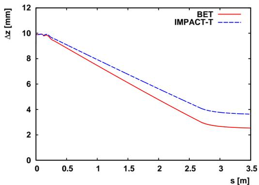
Figure 3: Evolution of bunch length in the two-cell capture cavity and the following drift space demonstrating ballistic compression.
