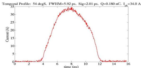
Figure 6: An example measured temporal profile at 135 MeV. The bunch was 0.72-mm rms in length (2.4 ps).
