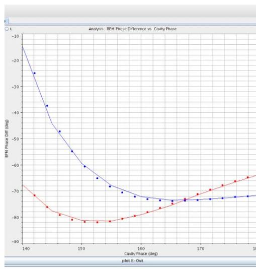
Fig. 1 The phase signature scan method result for a DTL tank (downstream BPM phase difference vs. DTL RF phase). Solid lines are measured, dots are model results, and red/blue represents different RF amplitudes. The nonlinear response on the LHS offers a unique "signature" for the model matching to meet.
