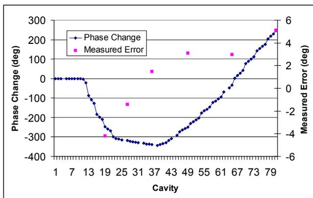
Fig. 4 Phase change (blue) resulting from reductions in 11 cavity gradients and activation of 1 previously unused cavity. Measured errors for selected cavities are indicated in purple.
