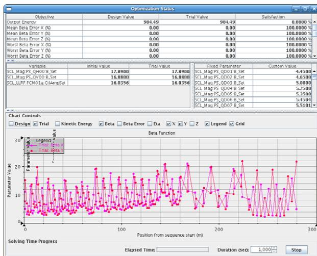
Fig. 2. A screen snapshot of the Energy-Manager application indicating some optimization figures of merits for matching, power supplies for variation and the resulting Twiss beta values along the SCL and downstream transport line.
