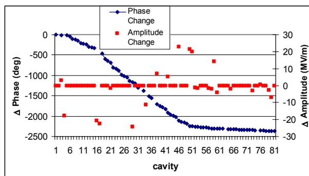
Fig. 5. Phase changes from the original beam based derived setpoints (blue) due to changes in the cavity gradients (red), predicted by the SLACS scaling technique.
