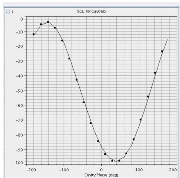
Fig. 3 Snapshot of an SCL phase scan. The downstream BPM phase difference is shown vs. the cavity phase over a 360 degree scan range.
