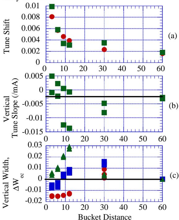
Figure 3: Tune shift, the tune slope and the spectrum width as functions of distance. (a) Tune shift at the bunch current of 0.5 mA, indicated by red dots (horizontal) and by green squares (vertical). (b) Vertical tune slope (mA), the black horizontal line indicates the measured tune slope at a single bunch. (c) Vertical width at bunch currents of 0.3 mA (green), 0.5 mA (blue) and 1.0 mA (red).
