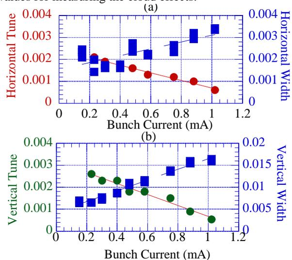
Figure 2: Horizontal tune and spectrum width (a) and vertical tune and the width (b) as a function of the bunch current measured at  $D=60$ . The tune is indicated by red or green dots and the spectrum width by blue squares. The tune of the head bunch of a train is used as the reference.
