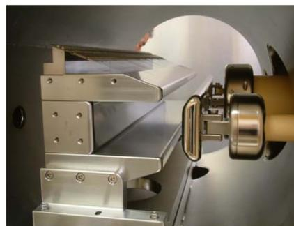
Figure 4: The thin septum ribbon mounted on the yoke of the half-length ESS model.
