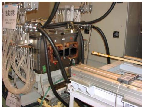
Figure 3: Field measurement of the fast-extraction septum magnets SM30.
