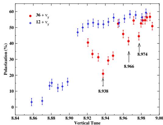
Figure 2: Polarization as function of vertical tunes at two intrinsic resonances with different resonances strength. The location of high order snake resonances near intrinsic resonances  $36 + \nu$  are marked.
