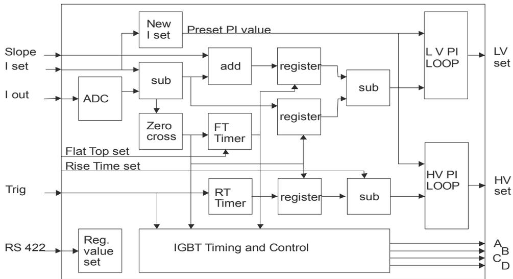
Figure 2: FPGA regulation loop
