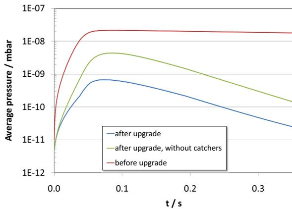
Figure 6: Evolution of the average pressure before and after the SIS18 upgrade.
