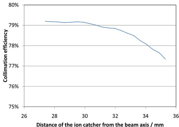
Figure 4: Catching efficiency for the process  $U^{28+} \rightarrow U^{29+}$  of the proposed SIS18 ion catcher system.
