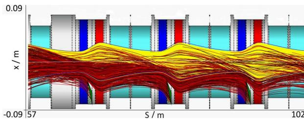
Figure 7: Tracks of ions after a charge change from  $U^{28+} \rightarrow U^{29+}$  in the horizontal plane of 4 cells of SIS100.
