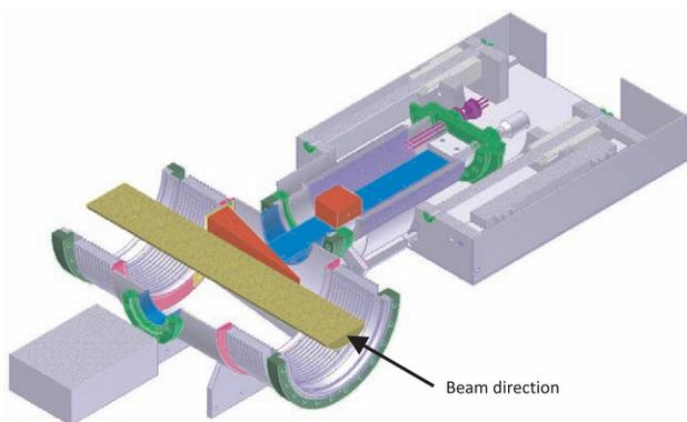
Figure 3: Design of the ion catcher system dedicated for beam loss by charge change in SIS18. A special wedge shaped collimator (red) design will be tested.
