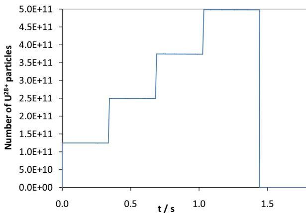
Figure 8: Evolution of  $U^{28+}$  beam intensity in SIS100 during stacking and acceleration.
