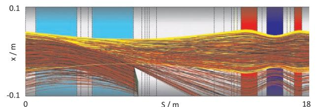
Figure 2: Tracks of ions after a charge change from  $U^{28+} \rightarrow U^{29+}$  in the horizontal plane of one cell of SIS18. Ion catchers are green, dipoles cyan, quadrupoles red and blue.
