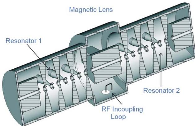
Figure 3: The coupled CH-DTL.
