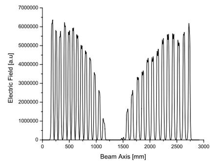
Figure 8: MWS electric field simulation for the first parasite mode of the second resonator of the FAIR proton injector.
