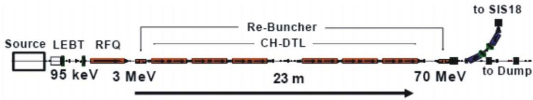
Figure 1: The layout of the FAIR proton injector.
