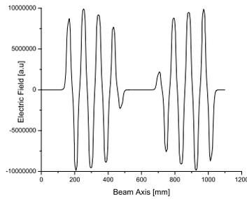
Figure 6: The electric field distribution for the  $\pi$  mode.
