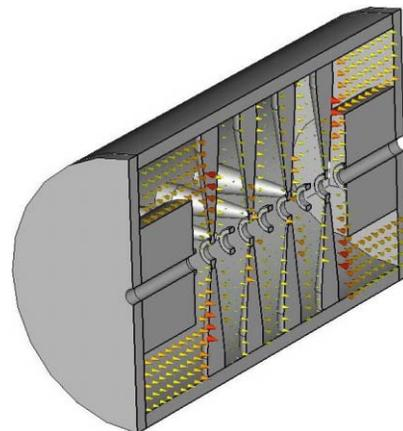
Figure 2: The magnetic field on CH-DTL's middle plane.
