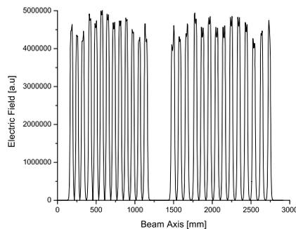
Figure 7: MWS electric field simulation for the second resonator of the FAIR proton injector.
