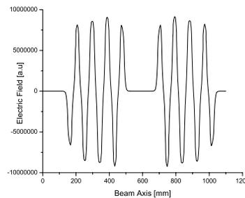
Figure 5: The electric field distribution for the 0 mode.
