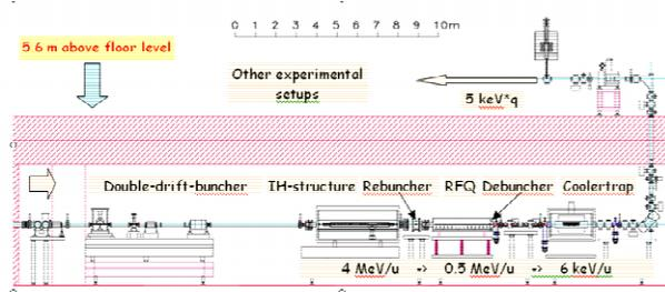
Fig. 2: Overview of the HITRAP-decelerator in the reinjection channel
