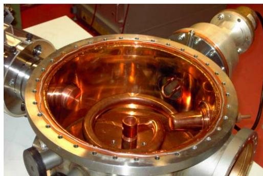
Figure 2: The Rebuncher-spiral-resonator with mounted plunger and coupling loop.
