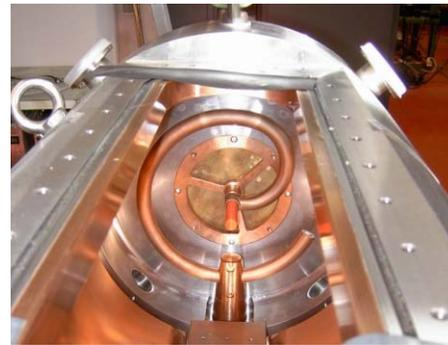
Figure 5: The Debuncher cavity before tuning and copperplating
