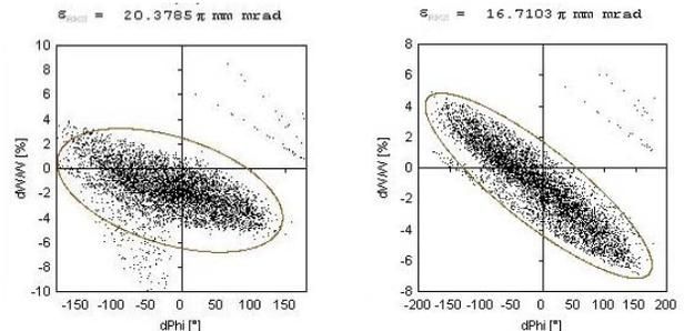
Figure 7: Output distribution with and without Debuncher.
